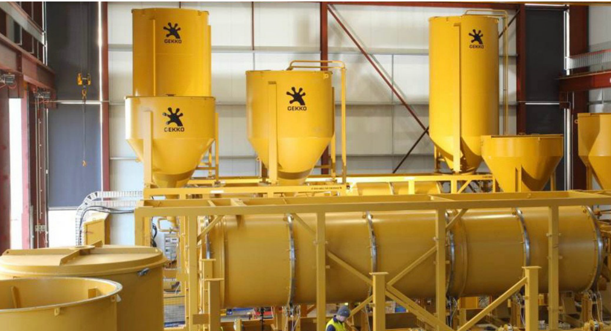
Figure 10: InLine Leach Reactor in the production shed in Ballarat, Victoria. All units are fully tested before shipped.
