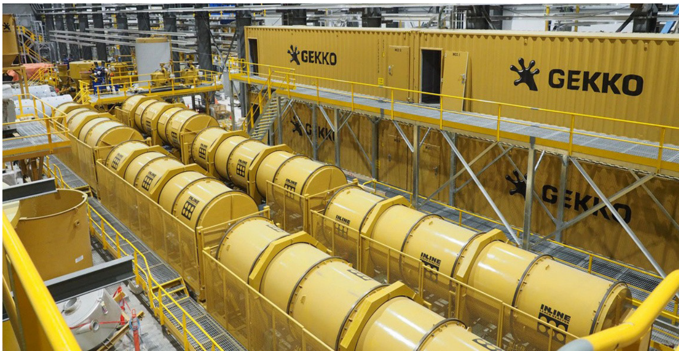
Figure 20: The ILR Continuous at the Hope Bay gold mine
