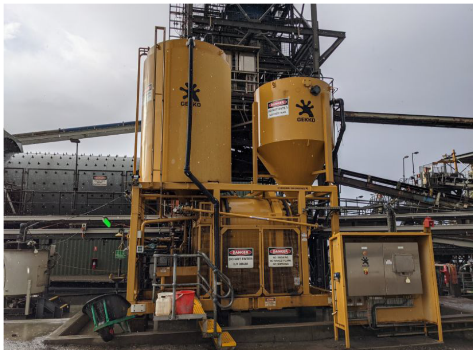
Figure 9: The ILR1000 Batch at Stawell Gold Mine. The ILR unit achieves +98 per cent recovery and is currently contributing 40 per cent of total gold production.
