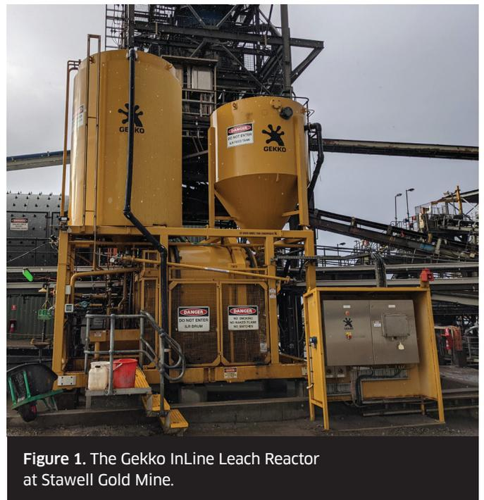
Figure 1. The Gekko InLine Leach Reactor at Stawell Gold Mine.
